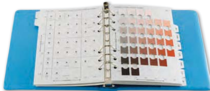
■ Figure 7.23 Hue, value, and chroma can be found using the Munsell System of Color Notation.
